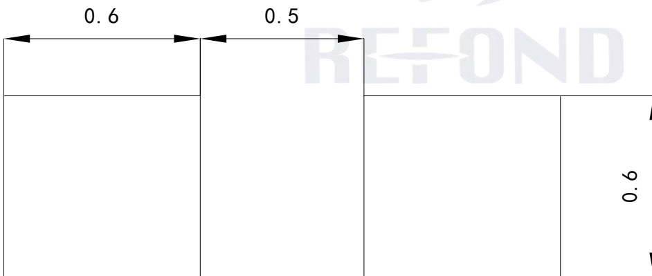
Fig.1-5 Soldering patterns 推荐焊盘
